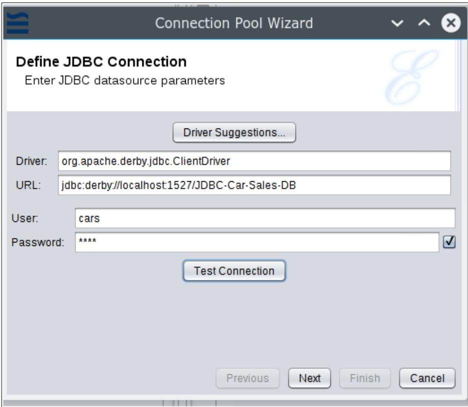
6. Click **Test Connection** to ensure that the connection works.
